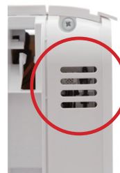
Sensor for indoor temperature and humidity
